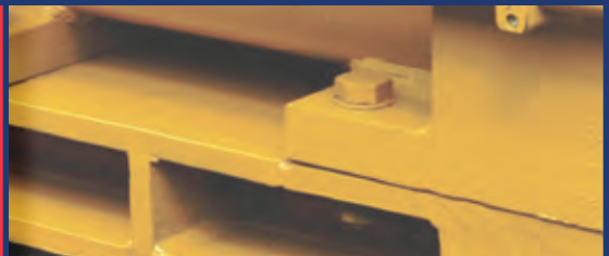
I-beam Foundation Base Plate
